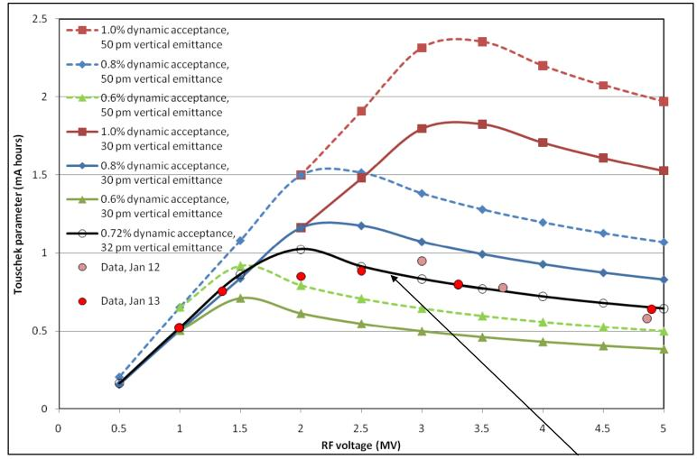
Measured energy acceptance =  $0.7\% \rightarrow \varepsilon_v \sim 32 pm$ From xBSM  $\sigma_v \sim 15\pm 5 \ \mu m \rightarrow \varepsilon_v \sim 38 pm$
