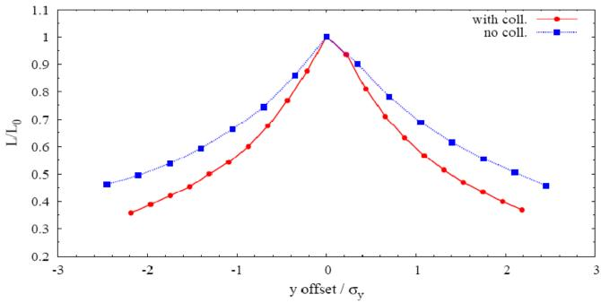
Jitter tolerance  $© 0.2 \sigma_v = 0.4 \mu m$  (  $\sim 10\%$  luminosity loss)
