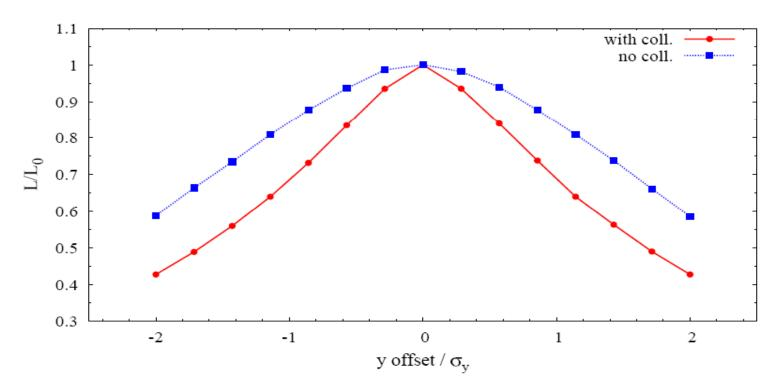
Position jitter tolerance  $0.2~\sigma_v \approx 0.1~\mu m~(\sim 10\%~luminosity~loss)$
