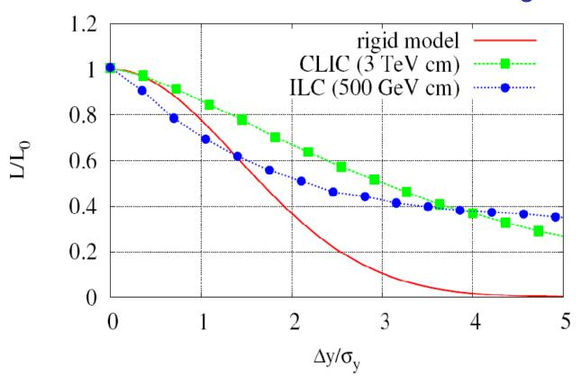
For instance, in order to maintain the luminosity 10% of nominal the relative beambeam position needs to be stabilised to within  $\bigcirc 0.5\sigma_v$  for ILC and  $\bigcirc 1\sigma_v$  for CLIC
