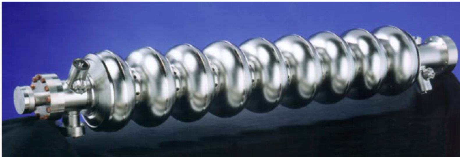
Figure 1.2-1: A TESLA nine-cell 1.3 GHz superconducting niobium cavity.
