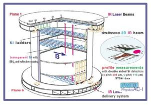
AMS-01 innovation (W. Wallraff) λ = 1082 nm IR "pseudotracks" 1-2 μm accuracy obtained Transmittance~ 50%
