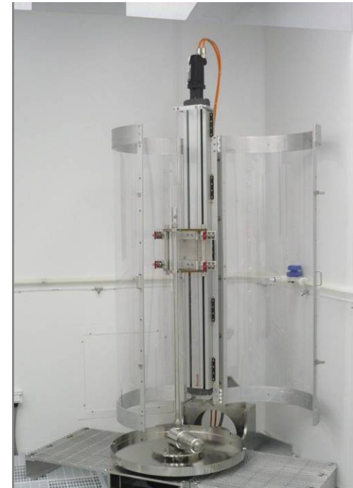
New High-pressure rinse system
