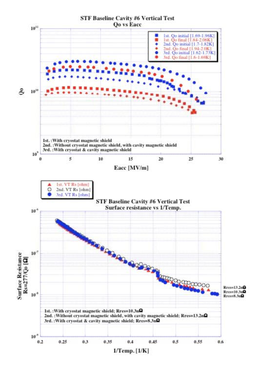
Q difference between 1<sup>st</sup> power rise and final power rise seems to be mag-field capture at quench.
