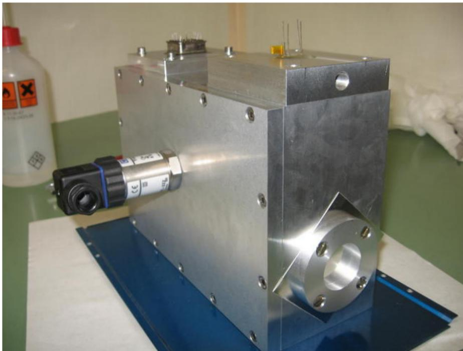
Closed prototype box, including the LED- & PM-mountings
