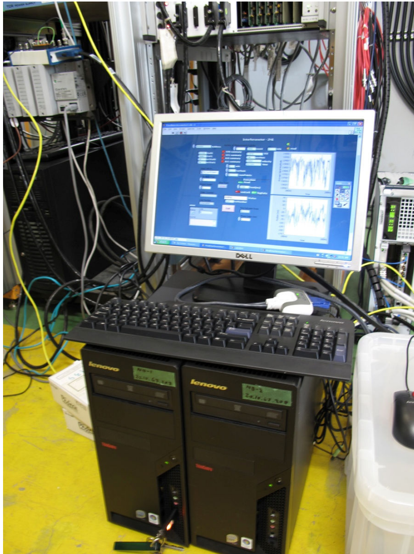
2 PCs, one for laser, one for CCDs
