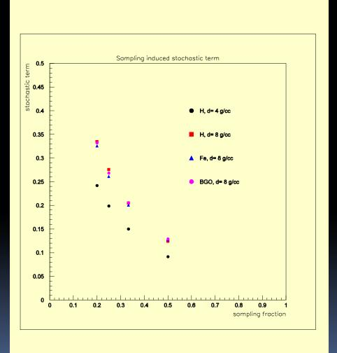
even a very large sampling fraction (30-50%) with sampling frequency of 1-2 cm induces a significant stochastic term in energy resolution • and it is a tip of the iceberg only. "Sampling fraction" is a function of particle type and particle energy. "Neutron problem" is a complete artifact of a sampling calorimeter with scintillator as an active medium, for example.
