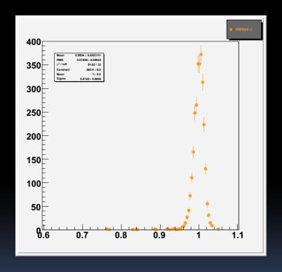
Use of the average correction degrades (slightly) the resolution: 1.38% instead of 1.22% and shifts the average response by 3.3%. The latter will induce significant degradation of jet energy resolution.
