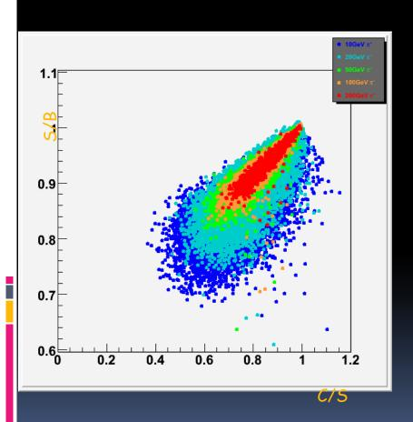
Correlation of the fraction of 'missing energy' and Cherenkov-to-scintillation ratio for showers of different energies: 10 - 200 GeV:
