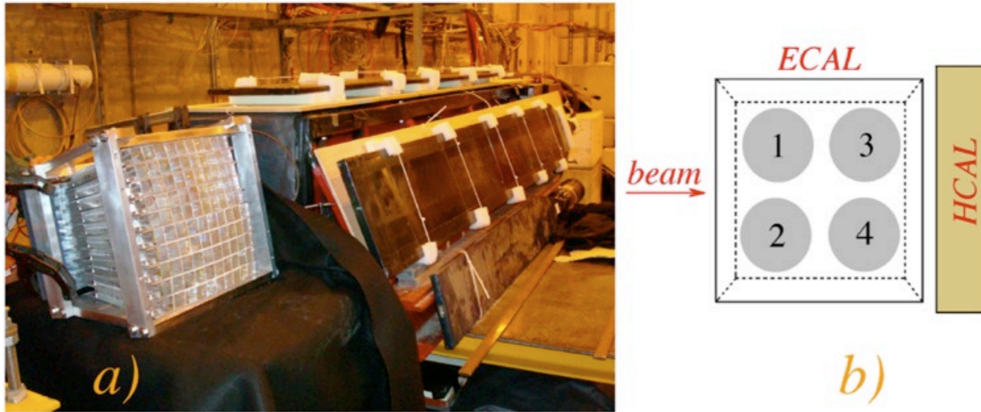
Figure 15: The calorimeter during installation in the H4 test beam, which runs from the bottom left corner to the top right corner in this picture. The 100-crystal BGO matrix is located upstream of the fiber calorimeter, and is read out by 4 PMTs on the left (small end face) side.
