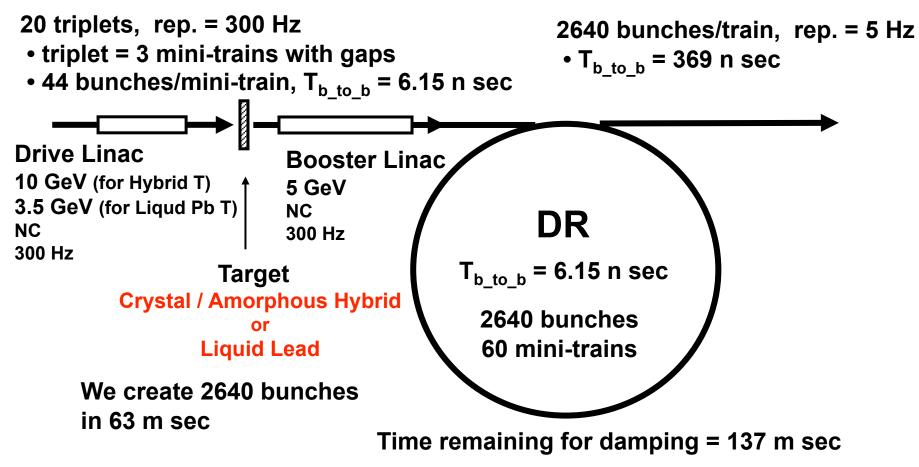
**e+ target R/D** Hybrid Target (Test at KEKB Linac)
