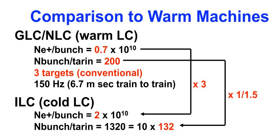
300 Hz generation: similar to warm machines in view point of target thermal/shock issues (diff = x2) Need 6 targets ?
