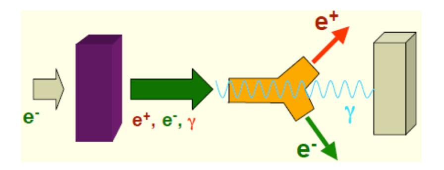
"Radiator" Thin CRYSTAL "Converter" Thick AMORPHOUS
