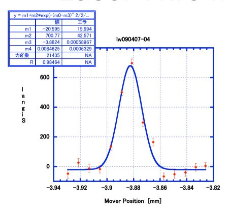
Minimum size measured=8.46um Measured Laser waist=5.96um → e beam size=~6um
