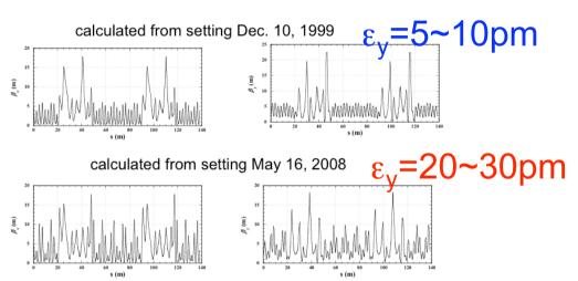
Kubo pointed out that the optics distortion is the one of the source of large emittance in DR.
