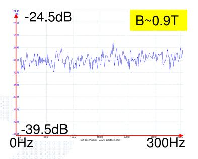
Data obtained from bearingmounted accelerometer with wheel operating at 800rpm.
