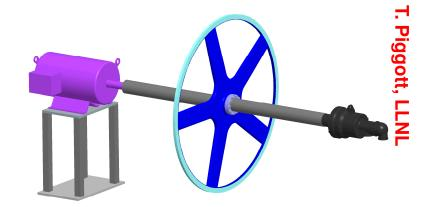
Drive motor and water union are mounted on opposite ends of through-shaft.
