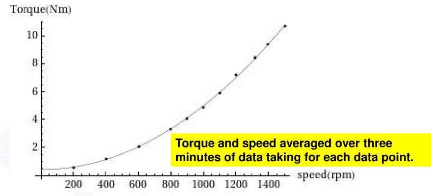
Data obtained with magnet off. Line shows quadratic fit to data points.
