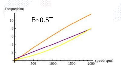
The plots show a quadratic fit to the measured torques (≤ 1200rpm) where the effects due to bearing friction have been removed.
