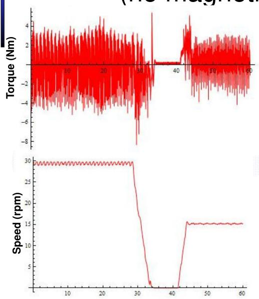
The upper figure shows the measured torque (Nm) as a function of time (s). The lower figure shows the measured speed over the same period of time.
