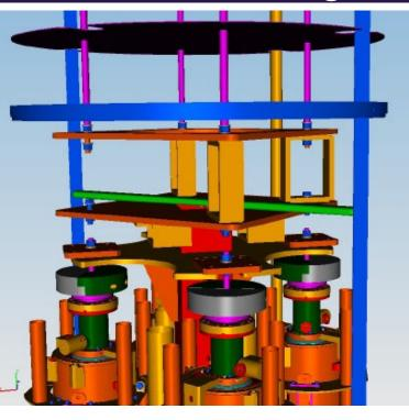
■4-cavity insert for AMTF test cryostats; design ready, construction a.s.a.p.
