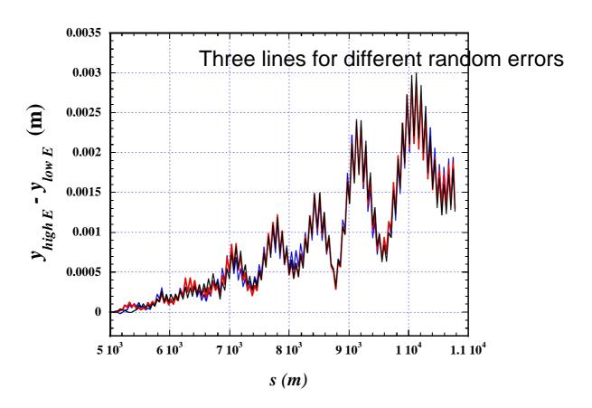
Orbit change by 2 mm at the linac end. No important dependence on misalignment.
