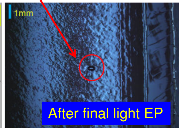
Defect in optical inspection picture of corresponding area of inner surface
