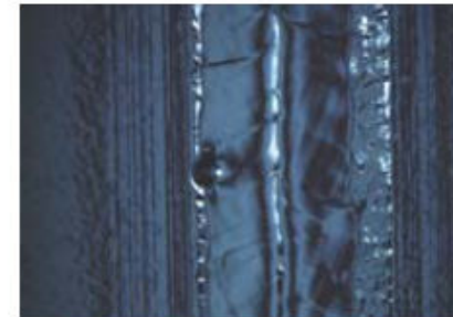
High resolution Kyoto-Camera. Spot on the equator of the cell 5
