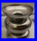
A rejected double dumbbell welded by AES was studied by JLab A natural weld spatter was identified and a 5  $\mu$ m BCP efficiently removes the spatter resulting a uniform surface finish
