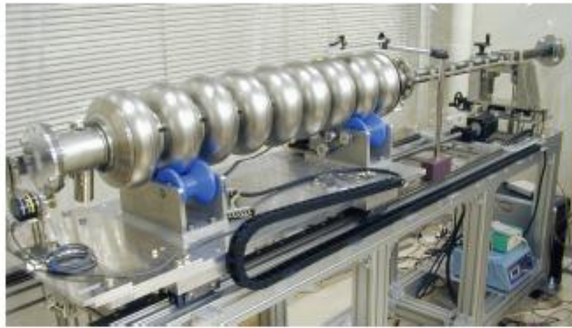
Camera system ( 7\mu\text{m}/\text{pix} ) in 50mm diameter pipe.
