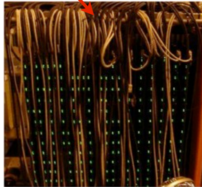
Analog HCAL 3x3 - 12x12 cm 2 lateral segmentation 38 layers, \sim 4.5 \lambda \sim 8 k channels
