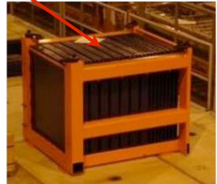
Tail Catcher / Muon Tracker 5 x 100 cm 2 Scintillator Strips 16 layers \sim 300 channels
