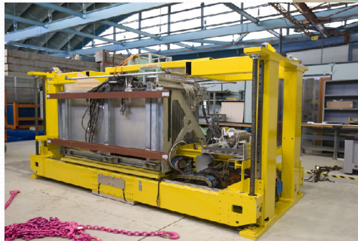
Construction ongoing, Beam test starts Spring 2010 Proof of principle for gaseous DHCAL
