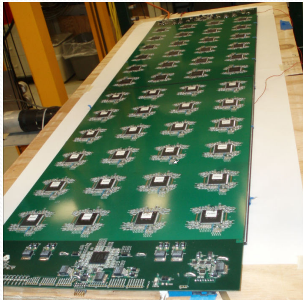
RPC checkup with 1\text{m}^3 electronics
