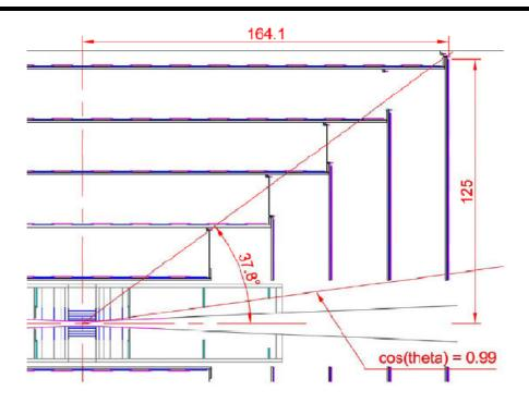
LOI geometry consisted of cylinders and disks with virtual segmentation
