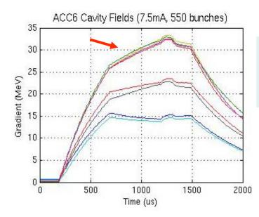
Substantial increase in gradient 'tilts' with 7.5mA (would have quenched with 800us flat-top)
