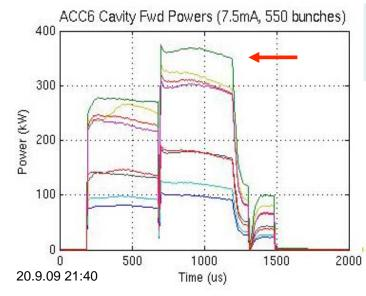
Power during flat-top is higher than the fill power for the 7.5mA case
