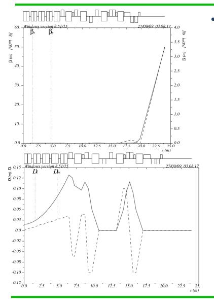
Taking the described approach to EL design, we obtain (in "linear"/"low energy spread" approximation): 24m long beamline with 17mm² beam size on the dump window. Dump is separated from the main beamline by 5.1m.
