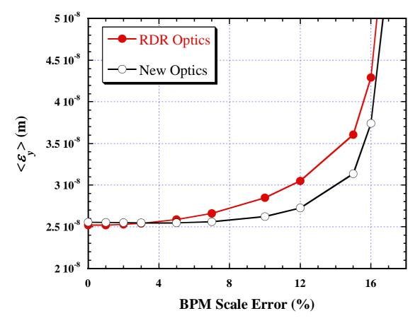
New optics is less sensitive to BPM scale error. But scale error > 10% will still cause a problem.
