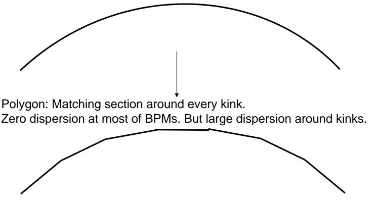
DFS for a polygon linac with 9 lines (8 kinks) was simulated.
