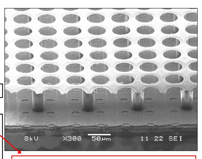
Now also Si<sub>3</sub>N<sub>4</sub> protection layers (7 μm<sub>2</sub>)
