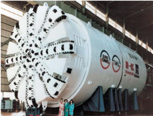
One of the world's largest tunnel boring machines. It has a diameter of more than 14 m.
