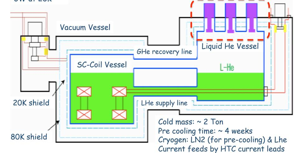
An example of semi cryogen free system SKS Cryogenics system at KEK
