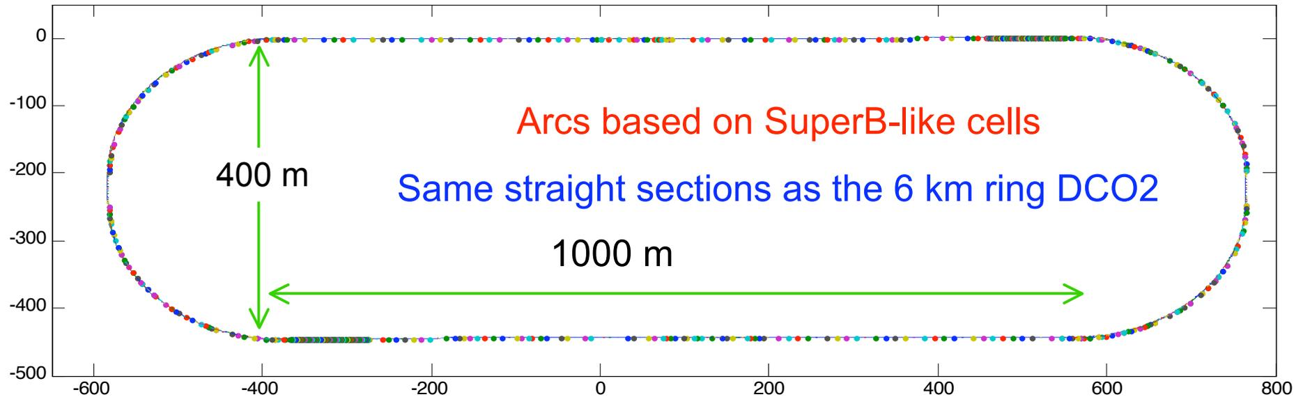
The lattice presented at LCWS08, Chicago has been updated to have injection extraction in the same straight section
