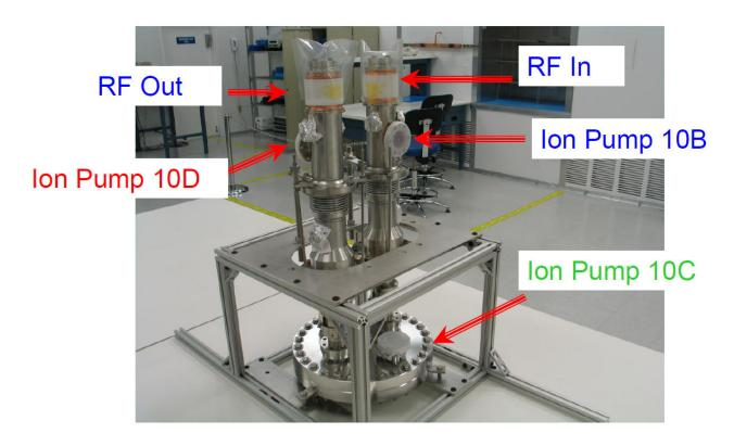
Power Couplers are high power cleaned, assembled and high power processed at SLAC
