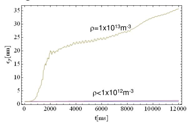
The interaction between the beam and the cloud is evaluated at 40 different positions around the DAFNE e+ ring for different values of the electoron cloud density.
