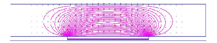
Simulation unsing POSINST code of electron cloud build-up and suppression with clearing electrodes. ILC DR positron: assuming one single 6 km ring.
