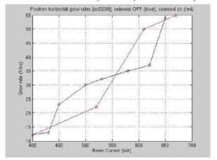
• Switching off the solenoids installed in the positron ring the grow rates of the e+ instability does not change
