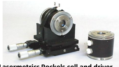
Lasermetrics Pockels cell and driver
