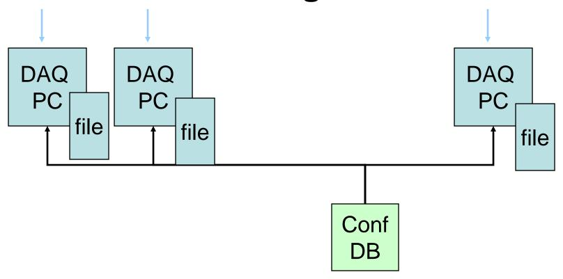
Extract conf files for all device servers from db, Recheck that configuration has been received
