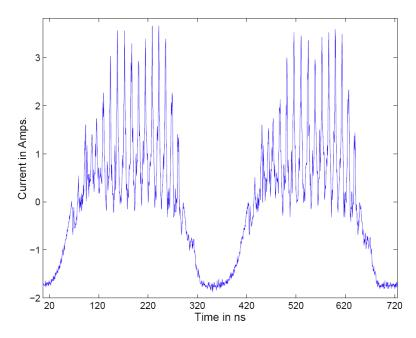
Observation of single-bunch longitudinal instability in the Los Alamos PSR, caused by an inductive impedance. From C. Beltran, A.A. Browman and R.J. Macek, "Calculations and observations of the longitudinal instability caused by the ferrite inductors at the Los Alamos Proton Storage Ring", Proceedings of the 2003 Particle Accelerator Conference, Portland, Oregon (2003).
