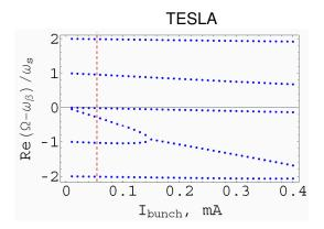
Calculations of TMCI thresholds in two designs for the ILC damping rings (by Sam Heifets). The bunch current at the nominal maximum bunch population of 2×10<sup>10</sup> particles is shown by a red line in each case.
