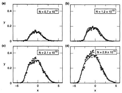
**Figure 6.4.** Potential-well distortion of bunch shape for various beam intensities for the SLC damping ring. The open circles are the measured results. The horizontal axis is  $x = -z/\sigma_{z0}$ , where  $\sigma_{z0}$  is the unperturbed rms bunch length. The vertical scale gives  $y = 4\pi e \rho(z)/V'_{rf}(0)\sigma_{z0}$ . (Courtesy Karl Bane, 1992.)
