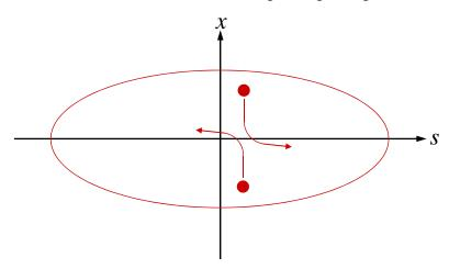
If the change in longitudinal momentum is large enough, the energy deviation of one or both particles can be outside the energy acceptance of the ring, and the particles will be lost from the beam.
