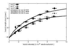
FIG. 5. Current dependence of the bunch length: Data are shown for the runs D', F', and E' (the symbols D', E', and F' indicate that the data were taken for the same condition as D, E, and F. but on another day.) The results of SAD simulations for 0.4%, 6%, and 3% coupling are superimposed.
