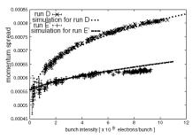
FIG. 4. Current dependence of the momentum spread: Data for the smallest (run D) and the largest emittance case (run E') are shown. (E' means that the data were taken in same condition as E, but on another day.) The results of SAD simulations for 0.4% and 6% coupling are superimposed.
