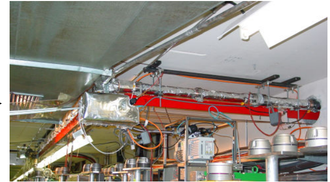
17m waveguide with 5 bends but low-loss (85% transmission) (Russian collaboration)
