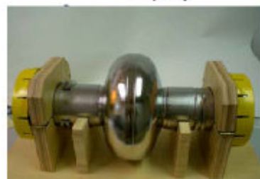
DESY single crystal cavity 1AC8 build from Heraeus disc by rolling at RWTH, deep drawing and EB welding at ACCEL
