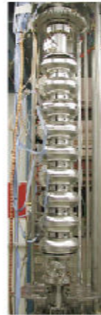
60mm-Aperture Re-Entrant Cavity, 58 MV/m! KEK/Cornell Collaboration
