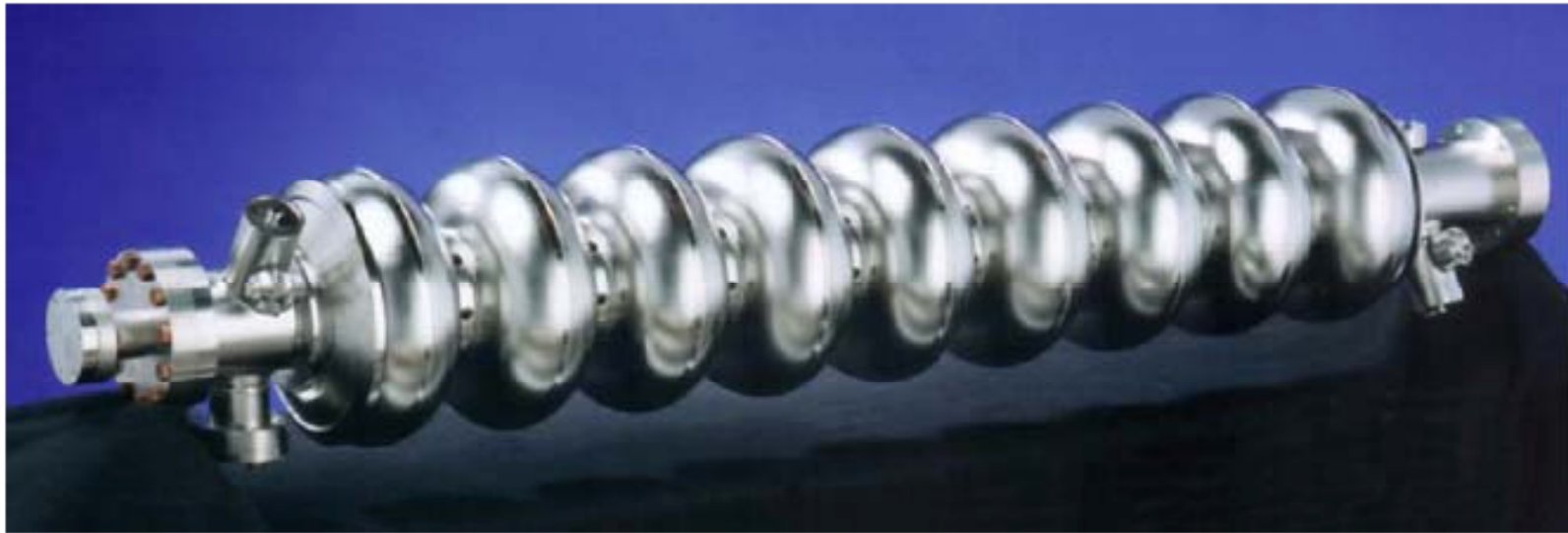
Figure 1.2-1: A TESLA nine-cell 1.3 GHz superconducting niobium cavity.
