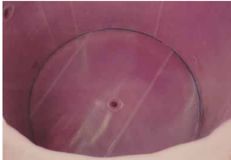
Teflon lining EP acid tank (brand-new)
