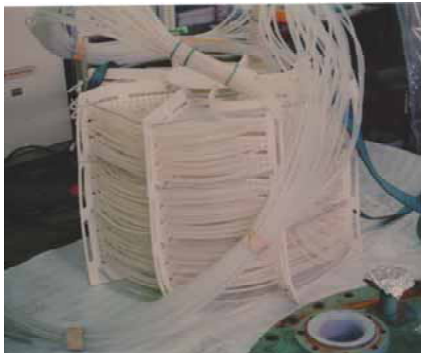
The contaminated heat exchanger
