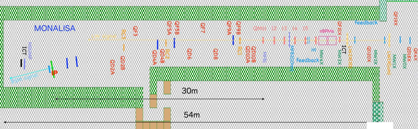
Shintake Monitor ( beam size monitor, BSM with laser interferometer ):Tokyo univ. MONALISA ( nanometer alignment monitor with laser interferometer ):Oxford univ. Laserwire ( beam size monitor with laser beam for 1 µm beam size, 3 axies):RHUL IP intra-train feedback system with latency of less than 150ns (FONT):Oxford univ. Magnet movers for Beam Based Alignment (BBA):SLAC High Available Power Supply (HA-PS) system for magnets:SLAC
