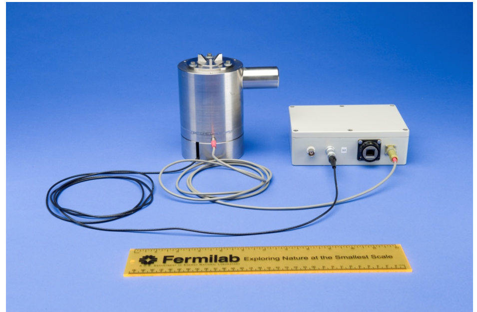
Ultra Sonic sensors power and signal over Ethernet
