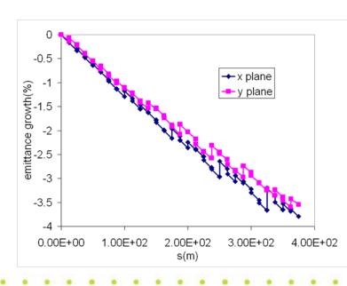
Undulator system damps emittance of drive beam by few %
