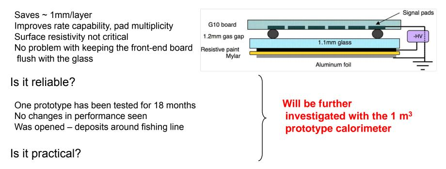
Once glued on, the front-end board can not be exchanged, without destroying the chamber
