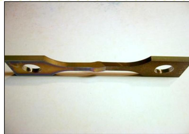
1. Ti-Ti joint samples welded by a company has pits at welded zone (both tensile test samples and impact test samples).
