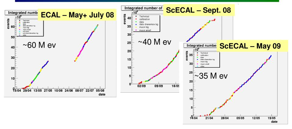
Smooth data taking after initial commissioning phase ~60 M events collected with Si-W ECAL + AHCAL (same as at CERN 07) ~75 M events with Sc-W ECAL + AHCAL (first time tested)
