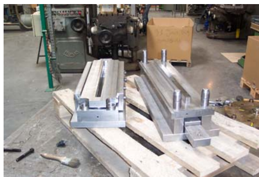
15mm thick plate with it's rails; ready to be assembled with EUDET's layers
