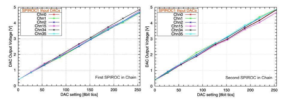
Both SPIROC1s show the same results. Output voltage **measured against +5V.**
