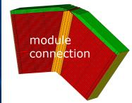
2 short length (360 mm) absorber sub-modules mounted to a short length module
