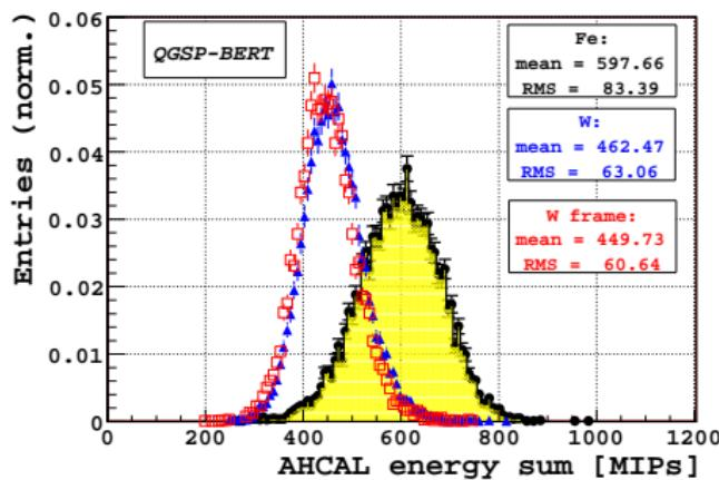
$\Rightarrow \sim 25\% (30\%)$  more energy deposited in case of Fe for LHEP (QGSP-BERT) than in W (more  $X_0$ 's in a W-layer)
