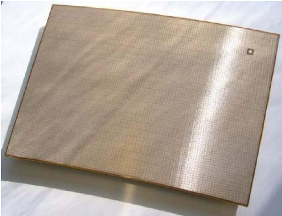
Standard bulk Micromegas module
